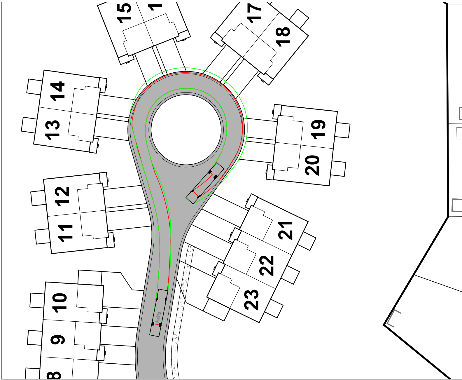
ROAD Q - FIRE TRUCK TURN MOVEMENT EXHBIT
